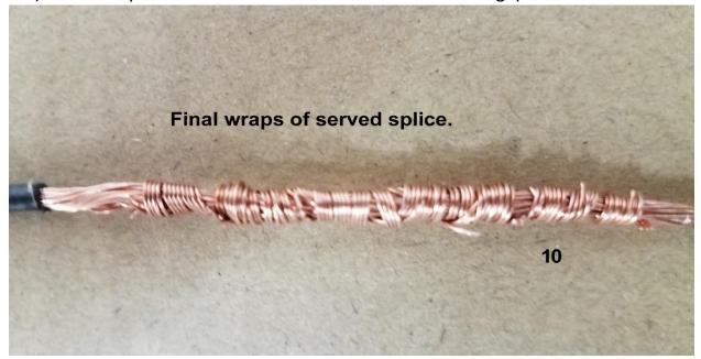
11.) I can pull with all my strength against a bench vice and the splice, even though not soldered, does not yield. It actually is a fairly good electrical connection. Of course, it is better soldered if the wire is not overheated and the solder is still flowed
