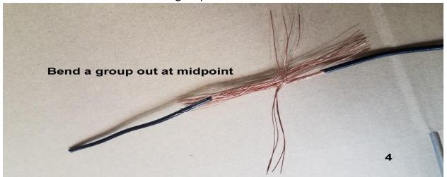
5.) Wrap the first groups tightly over all the other ungrouped wires, making a Western Union style wrap. Wrap until the ends are completely reached.
