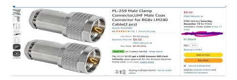
Dimension differences to standard UHF connectors are essentially the same except for length. The RG8X compression connector is very slightly shorter tip-to-nut length and slightly larger diameter than a standard PL-259 with RG8X reducer sleeve connector. This compression fitting will fit almost anywhere a standard UHF male will fit.
