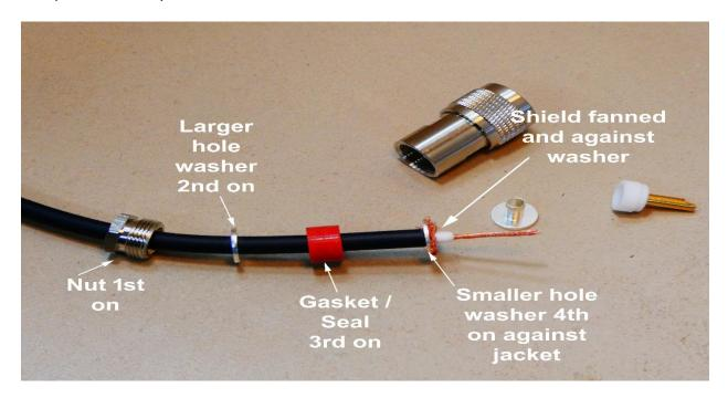
I prepped this cable by first cutting the center conductor to match pin length plus a bit:
