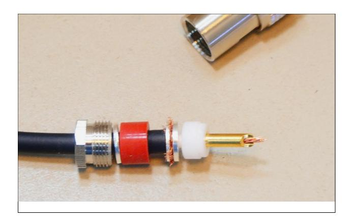
It is assembled and compressed now with wrenches. Hold the body steady and turn the nut!
