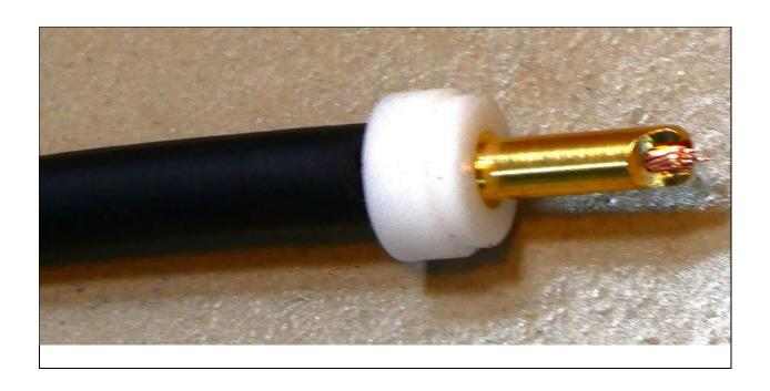
The insert is next and sandwiches the braid. No braid against gasket!
